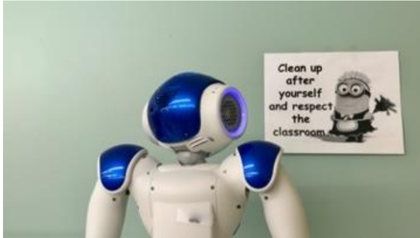
FIGURE 10 THE NAO ROBOT LEARNS TO VISUALLY CENTER THE OBJECT (THE PAPER SIGN) BY MOVING ITS HEAD.
