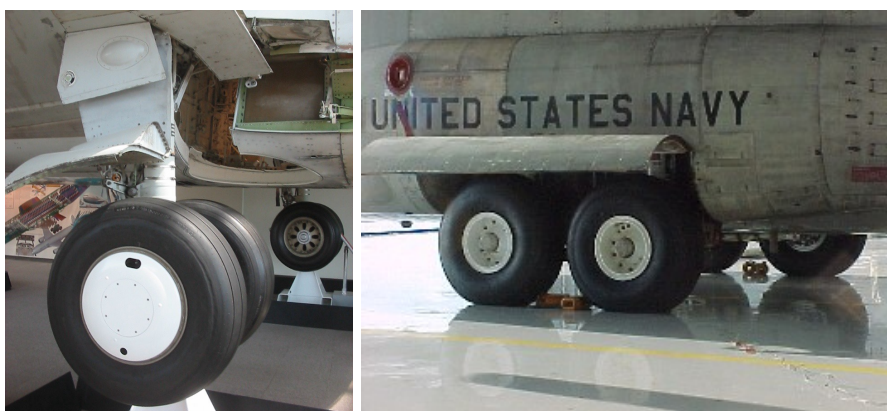
Figure 12-8. Landing Gear Retraction Mechanisms: Hydraulic Actuators (Left) and Fuselage Doors (Right)
