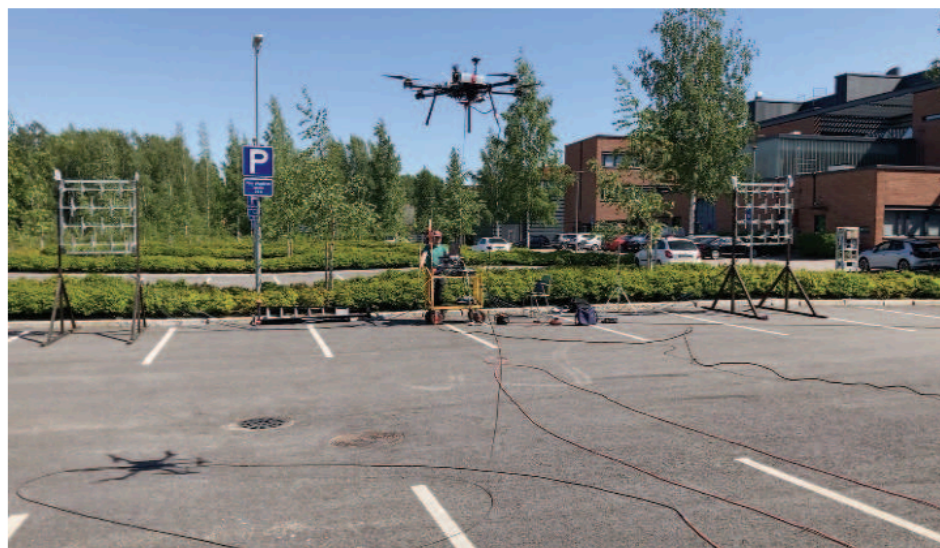
Figure 3. Antenna outdoor experimental setup
