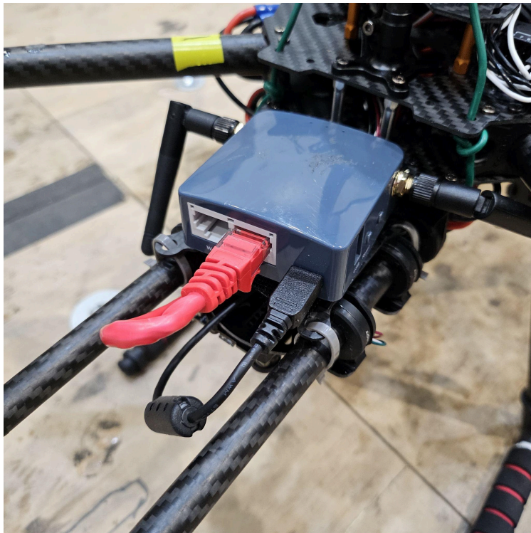
Figure 21. Onboard modem for Raspberry Pi
