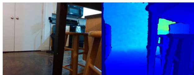
Fig. 3: Images provided by the RealSense D435 camera showing both an RGB image (left) and the depth view of the same scene generated by its depth cameras (right).
