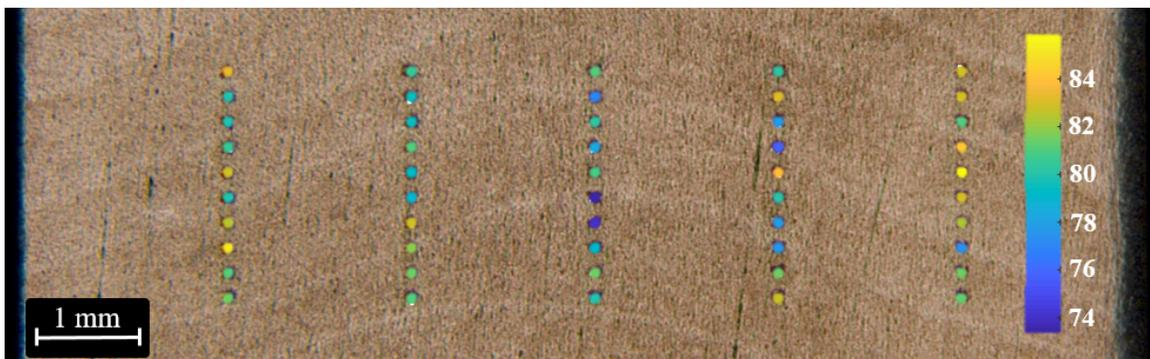
Figure 3.24: HV<sub>0.3</sub> of AD material sampling across deposit layers.
