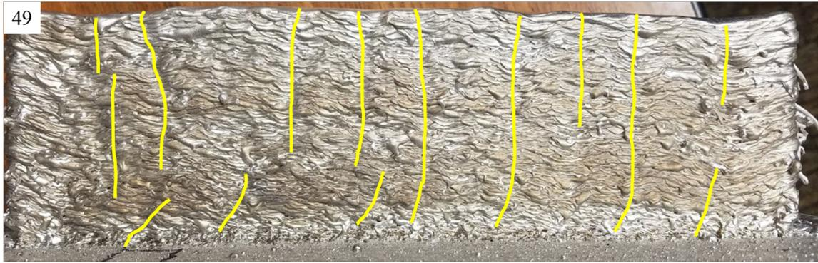
Figure 4.11: Image of the completed Plate 49 deposit, with macrocracks highlighted in yellow and widened for visibility.
