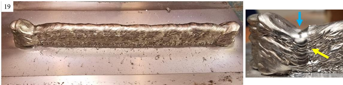
Figure 4.10: Image of the completed Plate 19 deposit. The inset shows an end of the deposit with slumping and cratering from the runbacks, as well as a macrocrack.
