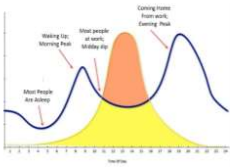
Figure 1: A general hourly grid energy demand curve (blue) and solar generation curve (orange/yellow) (Groves, 2019).
