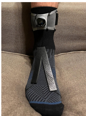
Fig. 2. Early-stage ankle brace prototype designed to address foot drop.
