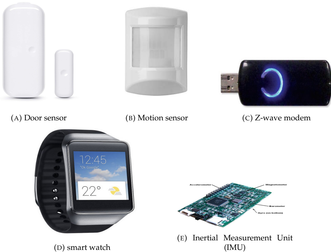
FIGURE 3.6: The first row shows Aeotec z-wave door sensor, motion sensor, and modem respectively by Aeon Labs. The next row shows Samsung Gear S smart-watch and an inertial measurement unit (IMU) with accelerometer, gyroscope, and magnetometer within the watch.
