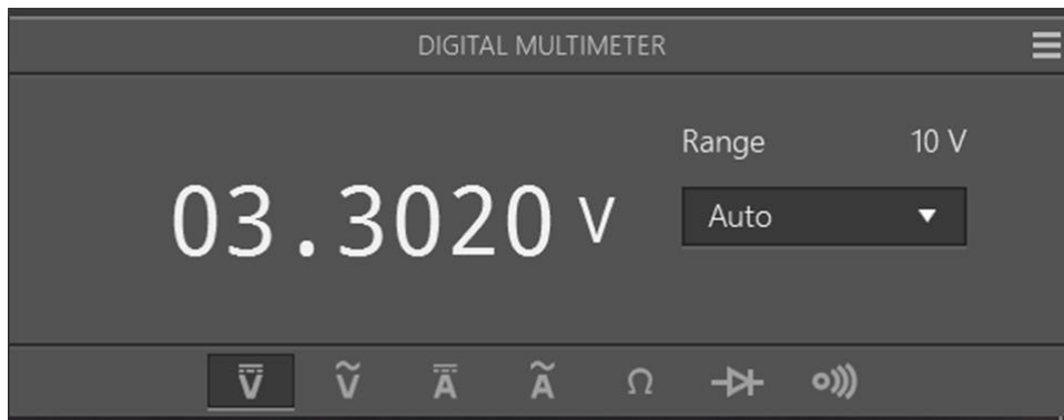
Figure 21: 3.3V Power Supply Verification (Remote)
