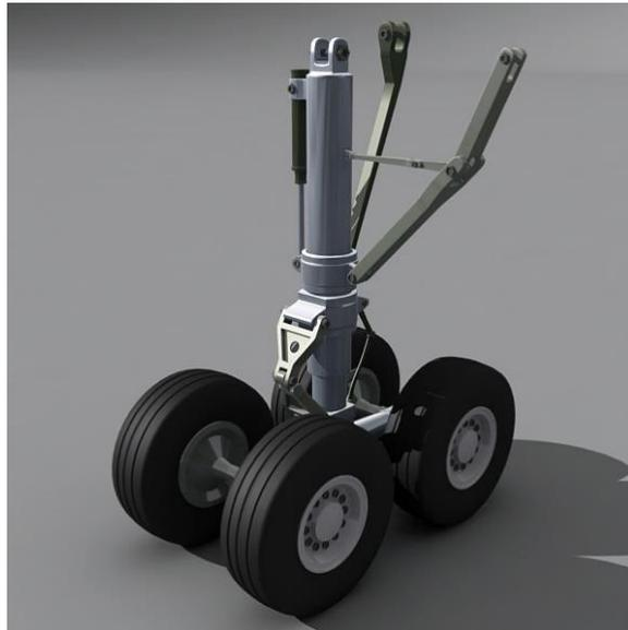
**Figure 39. Main Gear CAD Model**
