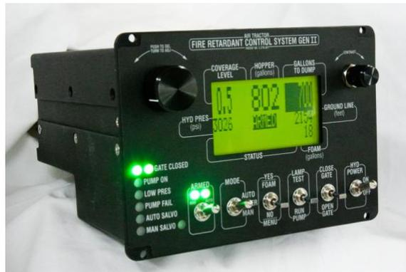
Figure 44. Fire Retardant Control System Gen II
