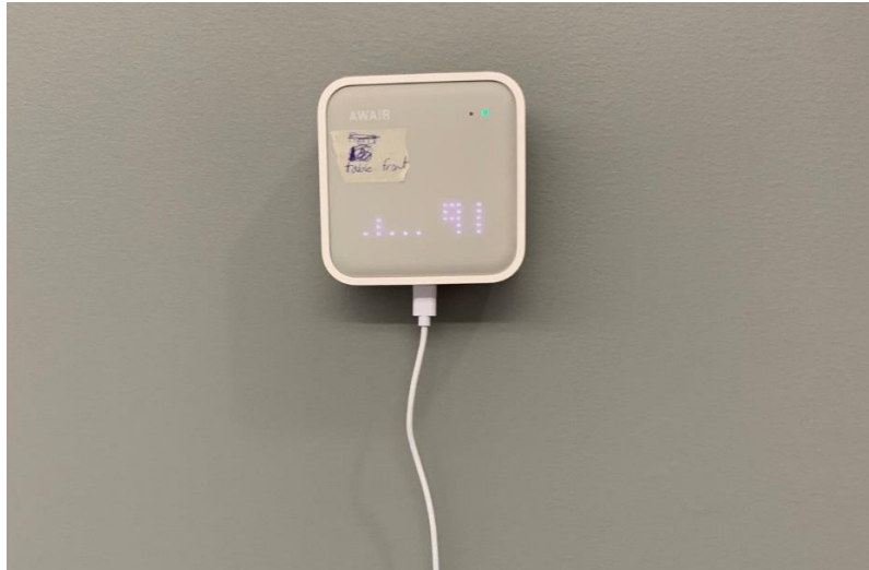
Figure 1: AWAIR Omni Air and Noise Quality Monitor to be used on the Contemplative Commons Construction Site
