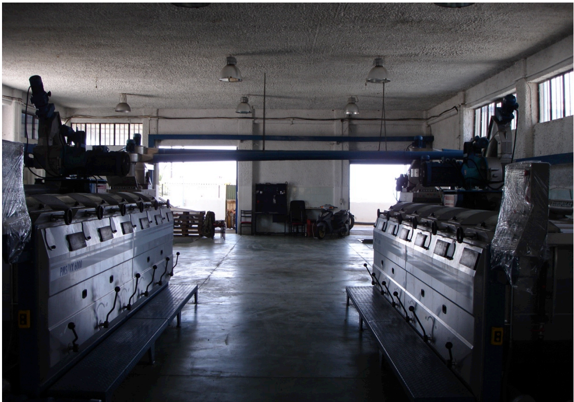
Figure 3-2. The oil mill in the off-season. Two banks of malaxers double the processing capacity.
