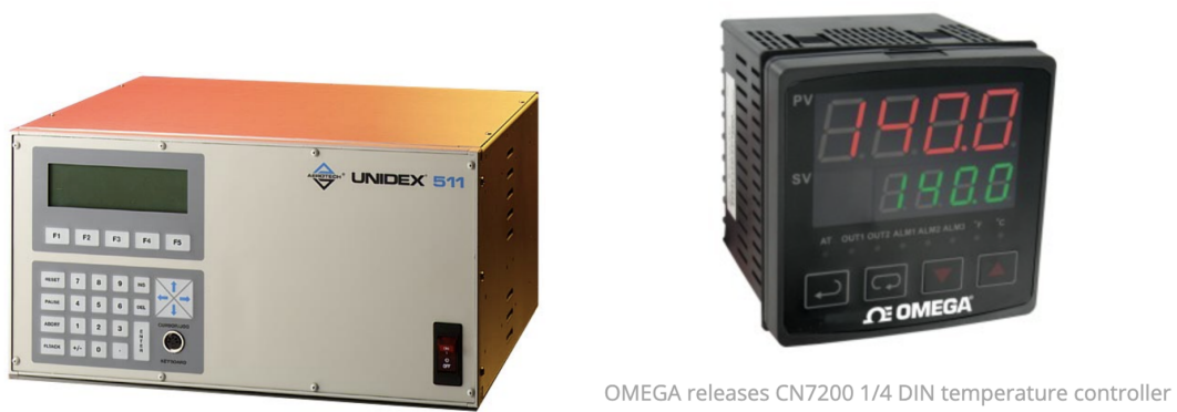
Figure 5.2: Motion controller and temperature controller for the Bridgman-Stockbarger growth.
