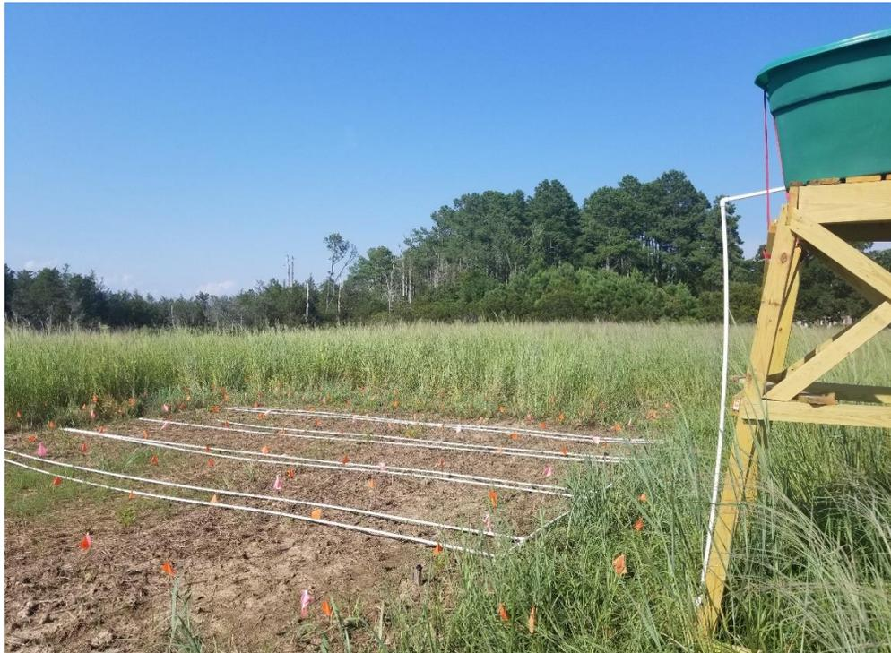
Figure 23. Water tower and irrigation system for the field experiment at the Brownsville Preserve in Nassawadox.
