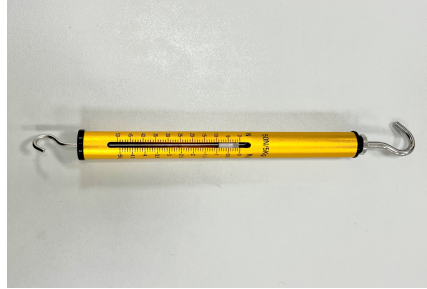
Figure 5: Spring Balance Used in Force Testing
