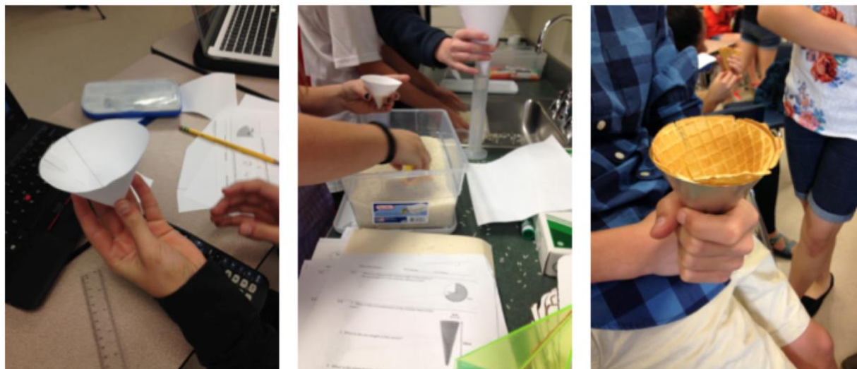
Figure 10. In the Ice Cream project, students created paper prototypes of cones, tested calculations by filling the cone with rice and measuring volume with graduated cylinders, and then created a metal prototype used to make an actual waffle cone.
