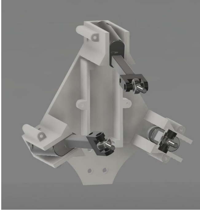
Figure 24. Final version of the base. This version improved joints and added the PCB cover.
