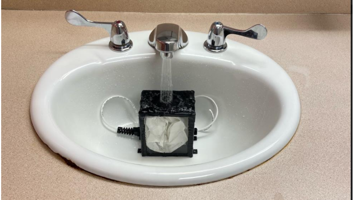
Figure 38. Back Box Waterproof Testing with Napkin
