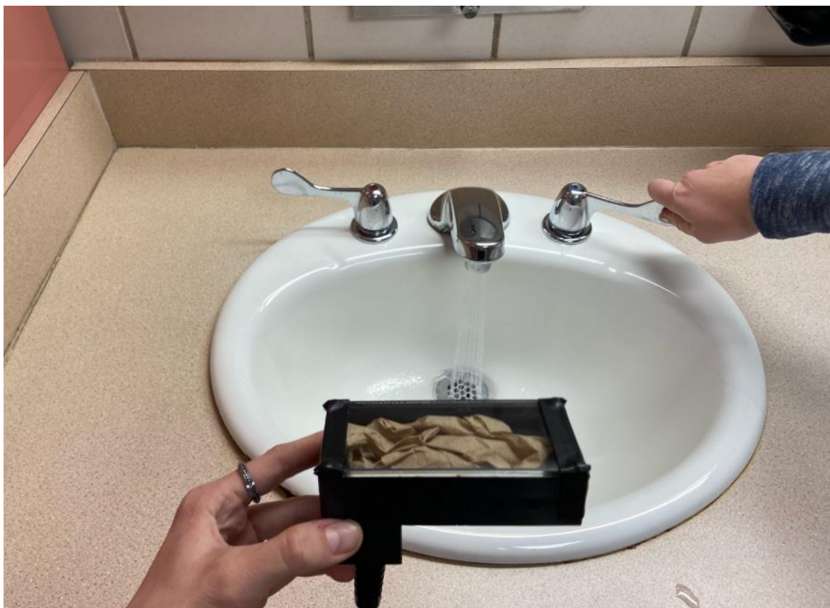
Figure 39. Front Box Waterproof Testing with Napkin
