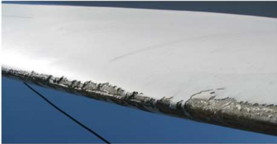
Figure 2. Leading Edge Erosion. Sourced from: Rempel L 2012 Rotor blade leading edge erosion—real life experiences Wind Systems Magazine
