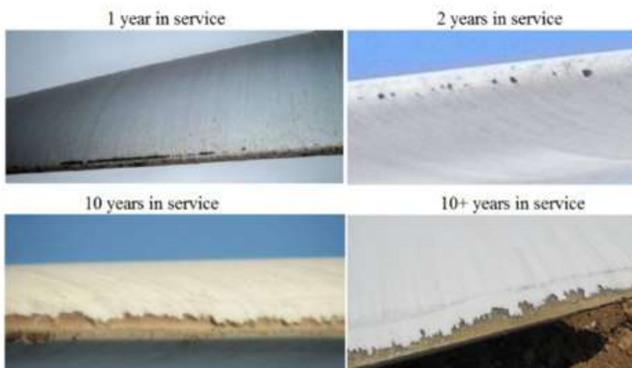
Figure 3. Leading Edge Erosion, Onshore Wind Turbines, Years in Service. Sourced from: Powell S 2011 3M wind blade protection coating W4600 Industrial Marketing Presentation
