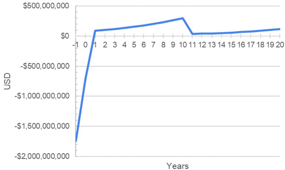
Figure 5.4-01: Scenario 1 DCF over plant lifespan
