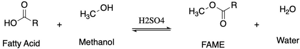
Figure 3.7-01: Esterification of free fatty acids into FAME.
