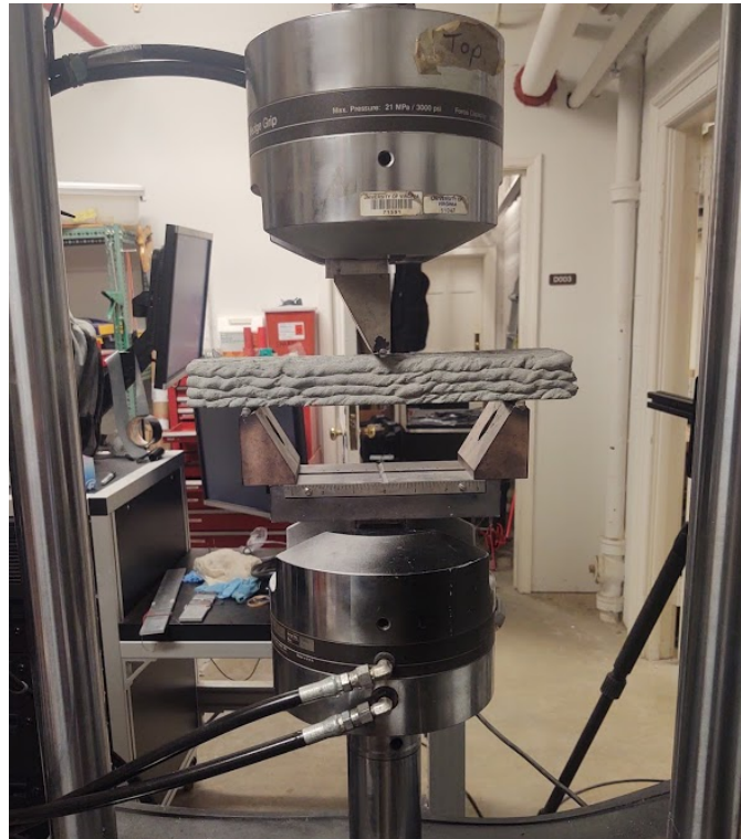
Figure 18: 3 Point Bending Flexural Testing Setup
