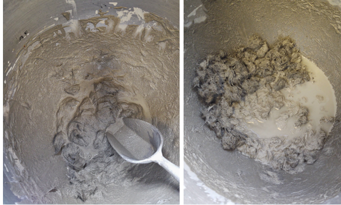
Figure 7: Photos taken of the M1 - VMA1+ANC1 - 2%PVA (left) and M2 - VMA1+ANC1 - 2%PVA (right) highlighting the clumping of the fibers after mixing.
