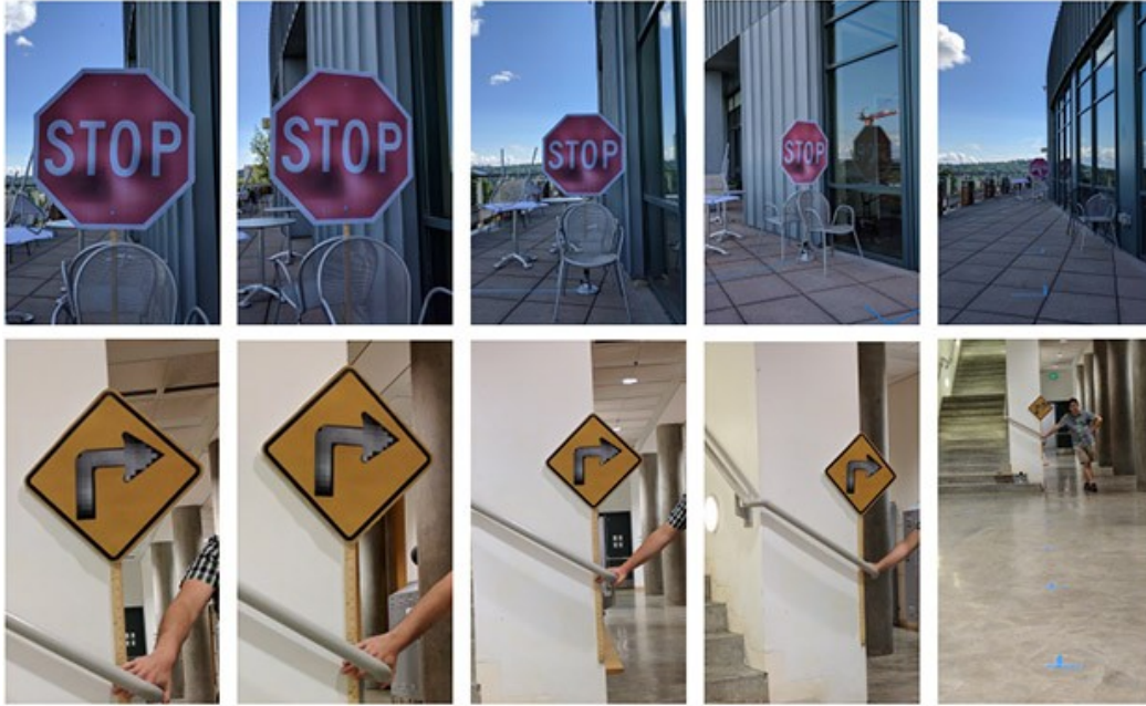
Figure 1. Examples of adversarial attacks on image recognition neural networks. The stop signs are interpreted as 45 MPH speed limit signs and the right turn signs are classified as stop signs despite relatively small changes to the appearance of the signs (Image source: Eykholt et al, 2018)
