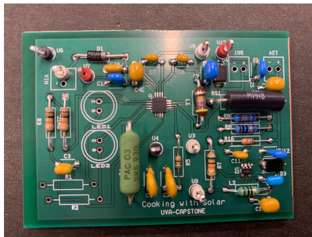
Figure 8: Soldered Solar Charger Controller PCB
