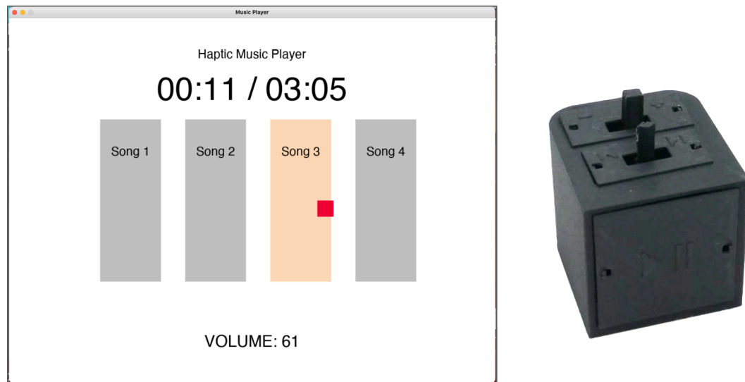
Figure 5.2: Music player app and PseudoWidget controller using Button on the front side and a lever and a knob on the top
