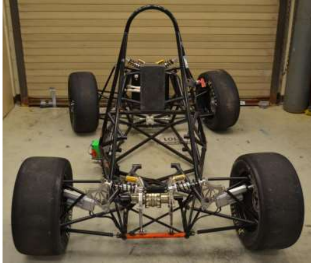
Figure 4. A RWPS design from the University of Washington’s FSAE team mounted into the vehicle’s frame. This image shows a rear view of the University of Washington’s RWPS design featuring independent electronic linear actuators in place of the rear tie rods to enable control over the steering angle of each of the individual rear wheels (Sparrow et al., 2016, p. 46).
