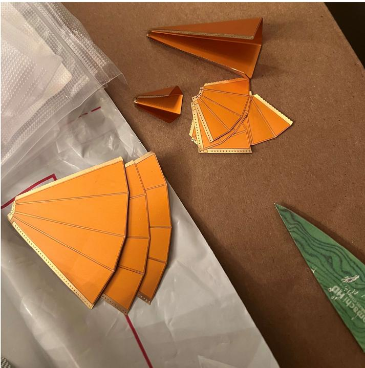
**Supplementary Figure 2 – Unfolded antenna templates.**
