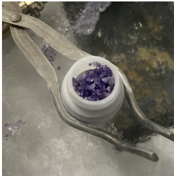
FIGURE 3.12: Ammonia irradiated using the new basket design. The dark purple color indicates that the desired dose for high polarization has been achieved.
