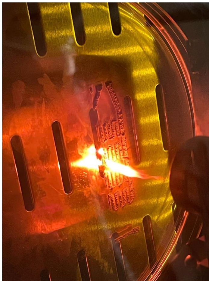
Figure 3: Laser Cutting of Mold: Laser cutting process of the mold, showing the intensity and precision of the cutting process. (Ghatnekar et. al. 2022)
