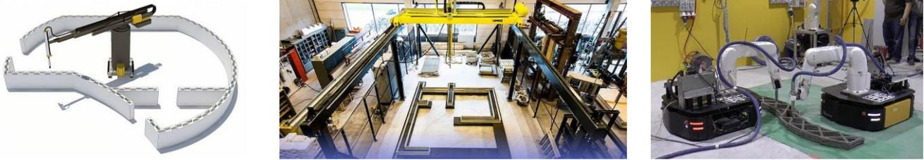
**Figure 8:** Concrete Printing systems. Left: Apis Cor crane printer diagram (apis-cor.com); Middle: Eindhoven University of Technology gantry printer (www.tue.nl); Right: Concrete printing robots (Zhang, 2019)
