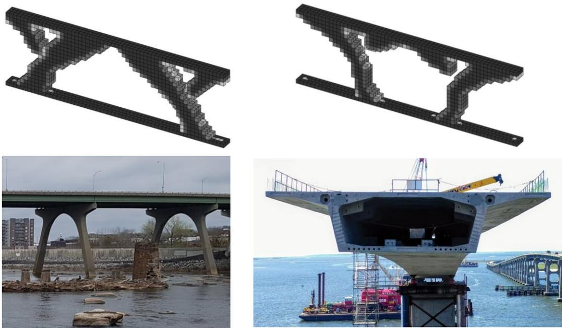
**Figure 46:** Comparison of SS-constrained hardened state wall results and common bridge designs. Top left: Table 12, Run 7; Top right: Table 12, Run 18; Bottom left: Bridge over the James River, Richmond VA (Photo by Seth Engel); Bottom right: Bonner Bridge box girder (Photo courtesy of HDR).
