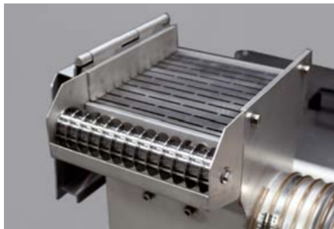
Figure 7.7.2 SE 400-2 Air Knife's Strand Guide and Split Sieve
