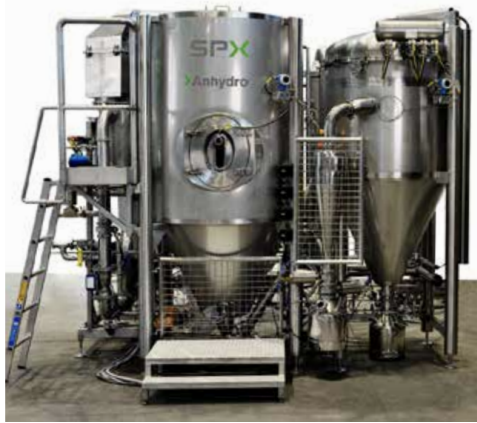
Figure 7.4.2. Pilot Scale SPX Anhydro Spray Dryer
