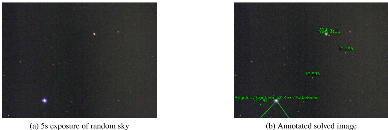
Figure 3.1: Annotated results of plate solving a captured image.
