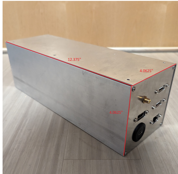
Figure 2.1: Enclosure with Dimensions
