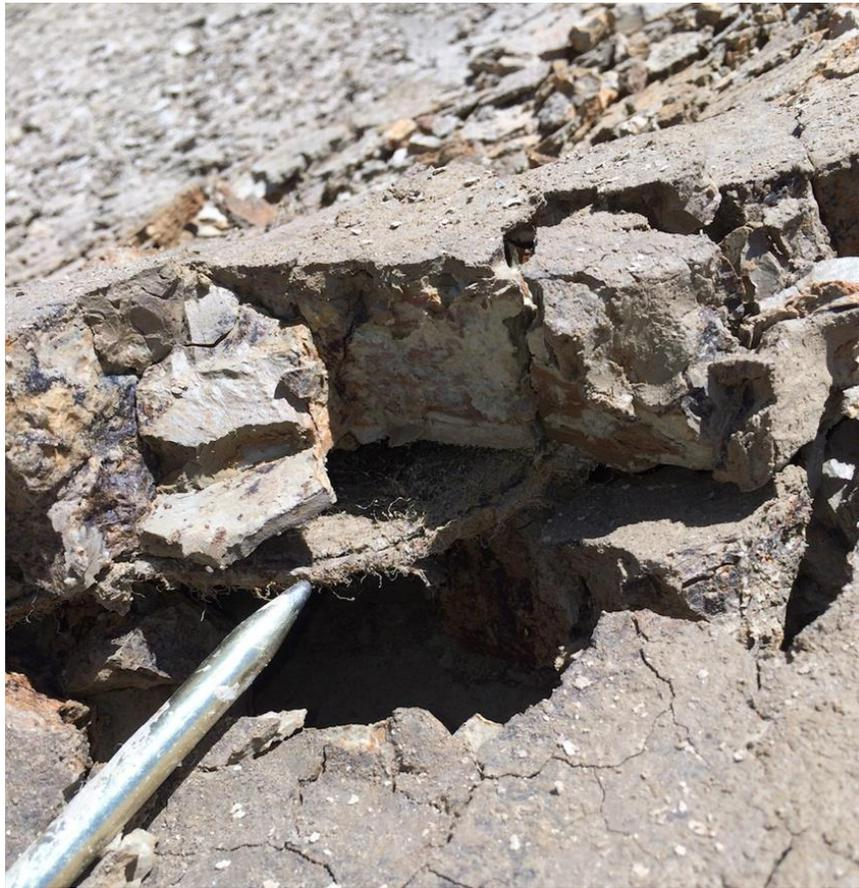
Fig. 4.5. Area of widespread material accumulation near the bottom of the slope, referred to as the "wedge". Material gathered above the GCL and underneath the GM. Image courtesy of Professor Jim Hanson at Cal Poly San Luis Obispo.
