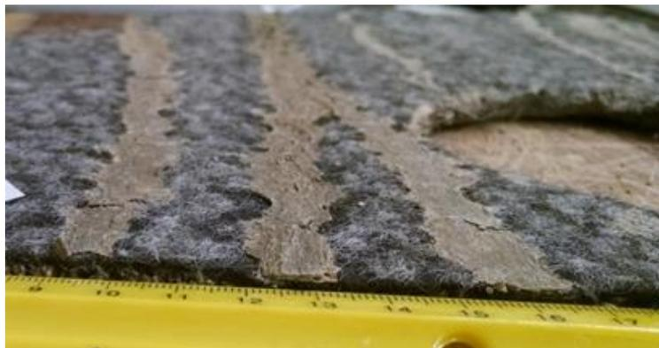
Fig. 4.3. Rivulets of eroded montmorillonite above GCL exhumed from the middle of the southeast corner slope (SE-M erosion rivulet).
