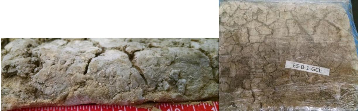
Fig. 4.4. Accumulation of bentonite near the toe of the east slope. The accumulated material lies above the GCL and below the GM. Accumulated material was not included in the mass per unit area measurements.
