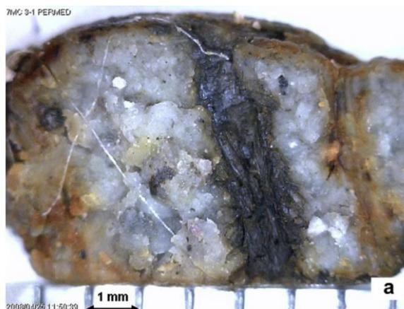
Fig. 2.6. Cross section picture of GCL interior before the addition of the dye, light area is hydrated bentonite, dark area is a bundle of needle-punched fibers along which preferential flow is suspected to occur, from (Benson et al. 2010).
