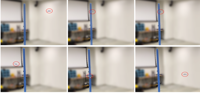
Fig. 12. Experiment for the recovery of the Crazyflie after colliding with a pole, showing the stabilization and replanning phases away from the POC.
