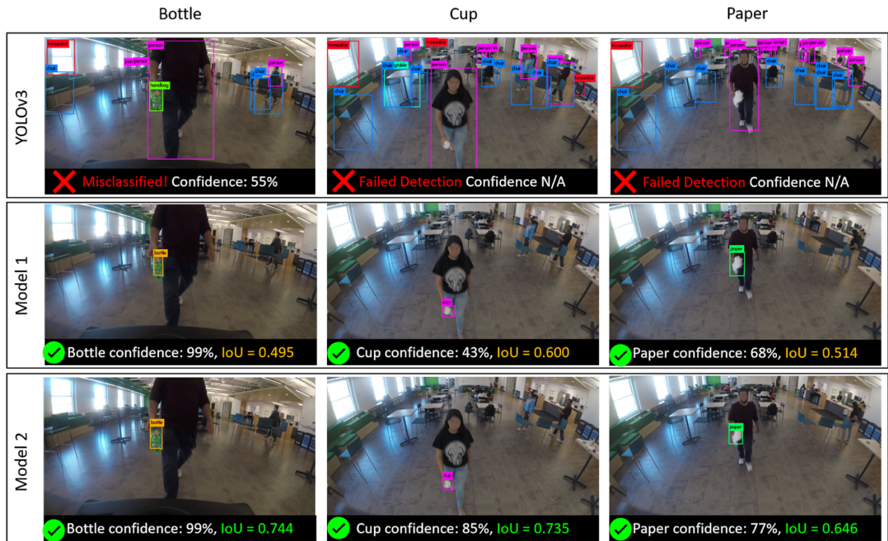
Figure 1. Examples of detection with output label, confidence, and IoU for each category.
