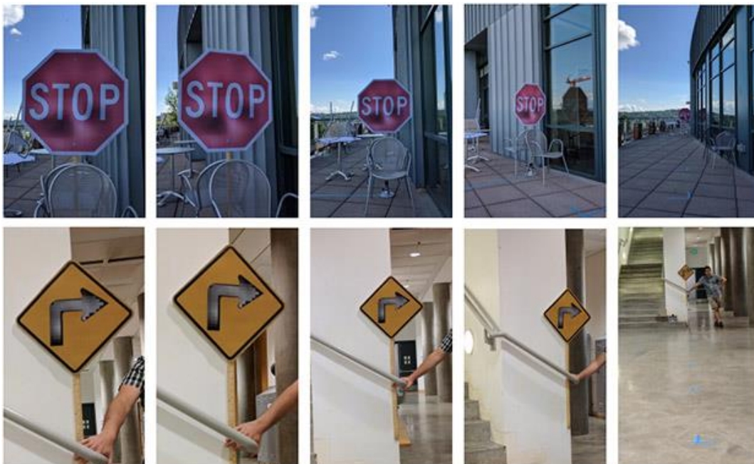
Figure 1. Examples of adversarial attacks on image recognition neural networks. The stop signs are interpreted as 45 MPH speed limit signs and the right turn signs are classified as stop signs (Image source: Eykholt et al, 2018)
