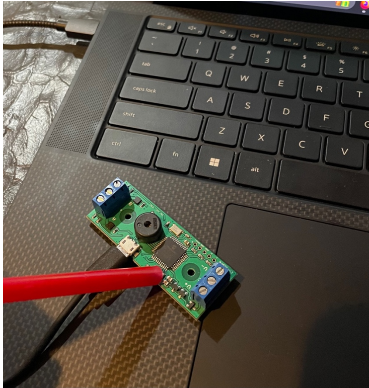
Figure 70. An example of the method used to simulate apogee during our tests that involved the Entacore AIM.
