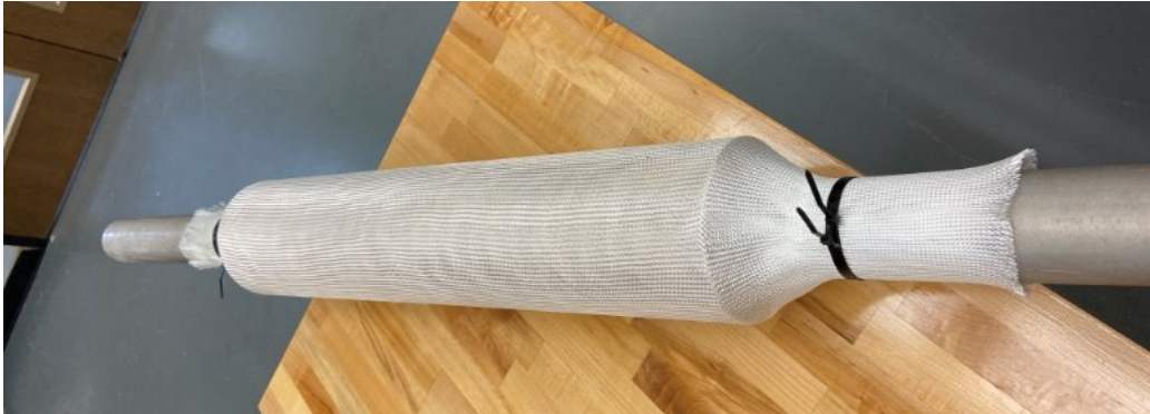
Figure 63. Fiberglass sleeve fixed over phenolic tubing.
