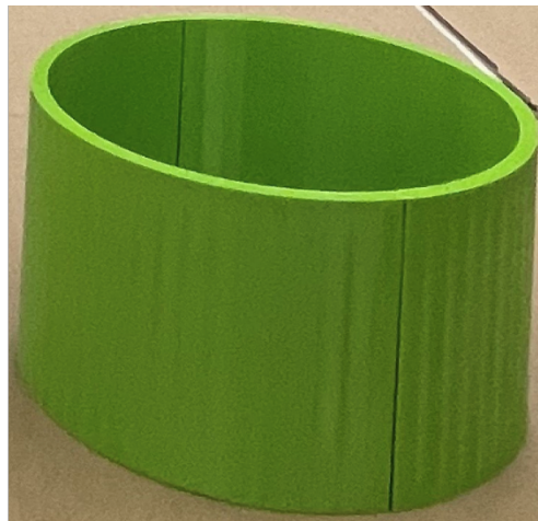
Figure 55. Extended nosecone mold (Height 10 cm)
