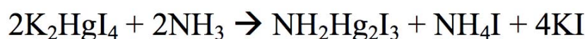
Figure 4-22. Chemical equation for the colorimetric reaction of ammonium with Nessler's reagent to produce a brown colored precipitate. Ammonia is produced from the reduction of ammonium with potassium hydroxide.
