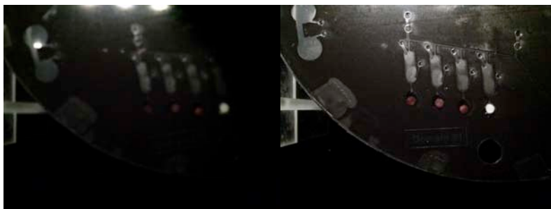
Figure 4-32. Image from the cell phone camera of the device without ( left ) and with ( right ) focus, with LED brightness adjusted using the power supply at 8.2 and 9 V, respectively.
