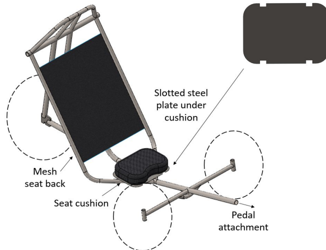
Fig. 1.10. Seat integrated into the frame design.
