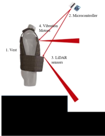
Figure 3: Side perspective of BAT. This figure depicts the locations of each component. (Tian, 2021)
