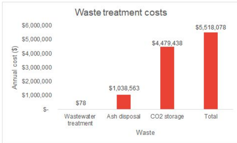
Figure 7.1-2: Breakdown of waste treatment costs
