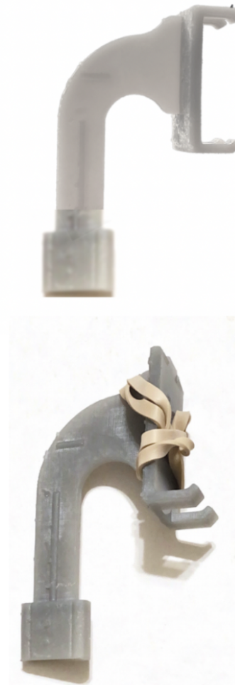
Figure 2. Novel positioning device: This is the device that we designed, 3D printed, and used for our testing trials.
