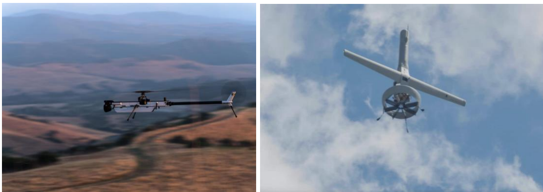
Figure 1: Left, Anduril Industries' advanced GHOST autonomous sUAS (Pondella, 2020). Right, Shield AI's V-BAT vertical-takeoff-or-landing (VTOL) UAS (Tseng 2023).
