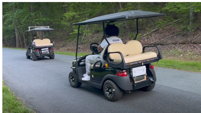
Fig. 1: Golf Carts Platooning on Straight Path
