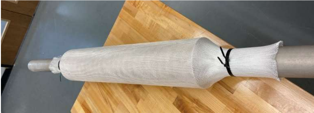
Figure 63. Fiberglass sleeve fixed over phenolic tubing.
