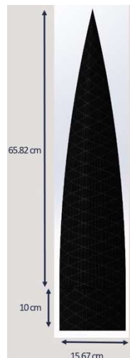
Figure 3. Final ogive nosecone design and dimensions.
