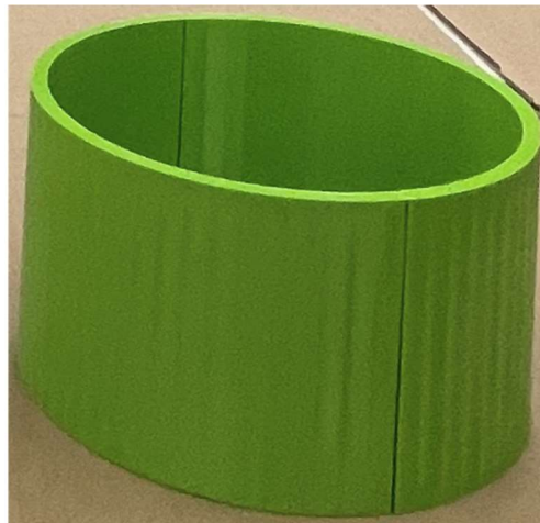
Figure 55. Extended nosecone mold (Height 10 cm)
