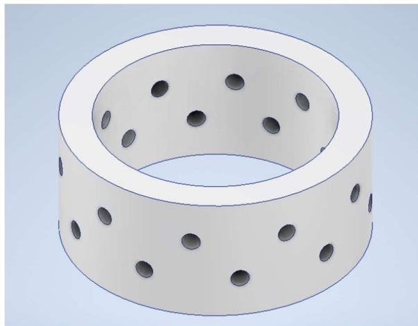
Figure 38. 2 nd Nozzle Holder Design
