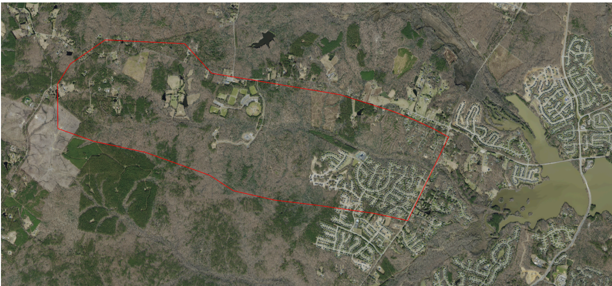
Figure R2.1. Topographic GIS Drainage Area Delineation
