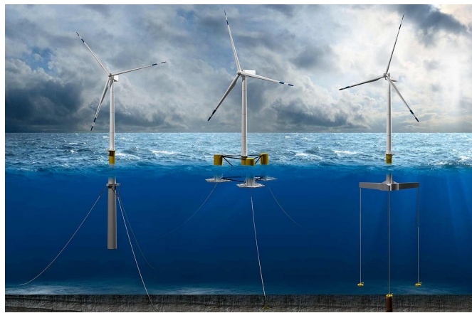
Figure 1. From left to right: Spar-buoy, Semi-submersible, Tension-leg platform.
