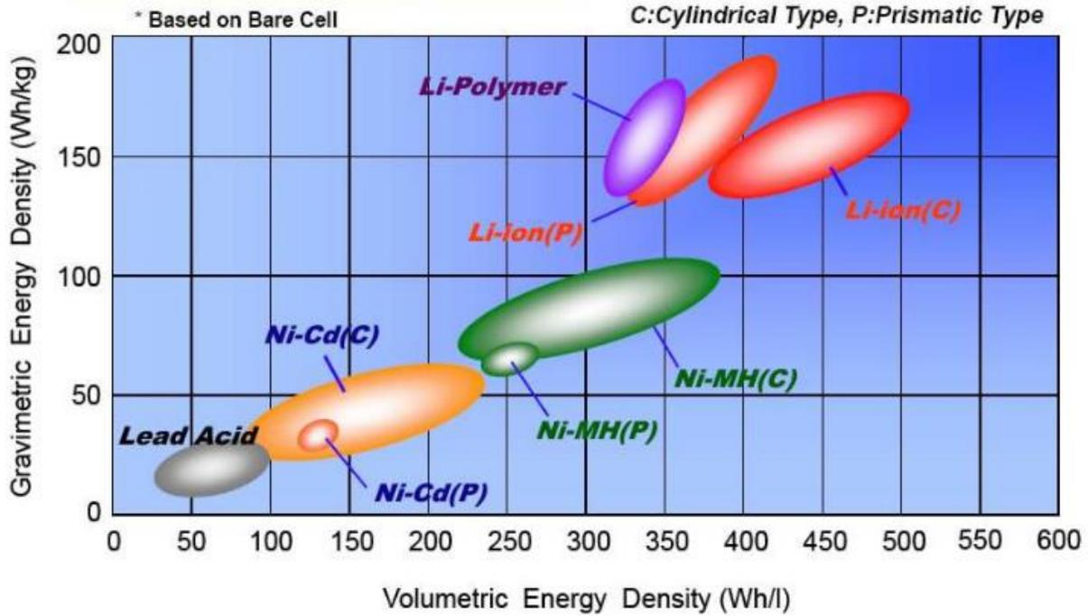
Figure 7: Battery Chemistry Comparison Graph (NASA Ames)
