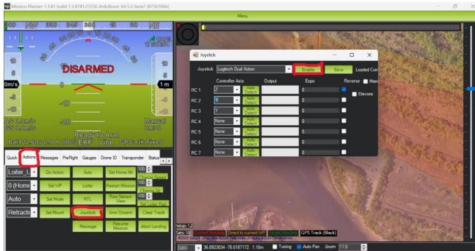
11. To arm, press the start button on the gamepad controller, OR click the Arm/Disarm under “Actions” tab in Mission Planner. For throttle input to go forward or backwards, go up/down on the left analog stick. For steering, go left/right on the right analog stick and the rudder should move.
