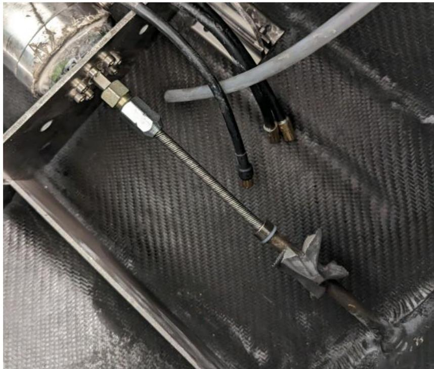
Figure 26: Flexible Shafts Installed and Connected to Motors
