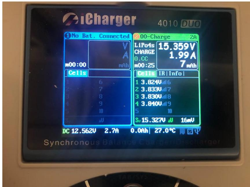
**8b.** If you are not satisfied with the amps: click the “Tab” button to switch from confirm mode to choose mode, and use the big wheel to choose the amps. Press the big wheel down to select the amps, then use the wheel to adjust. Reverse this process to go back to the Charge option and start charging.
