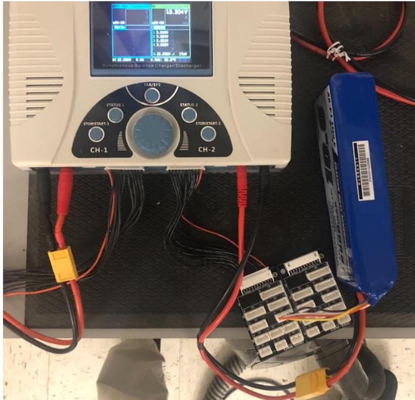
6. Setup the charger: There are two sides, make sure you are using the correct side using tab, it will highlight which side you are “working” on. You can use the buttons, the big scroll wheel, and press down on the scroll wheel.
