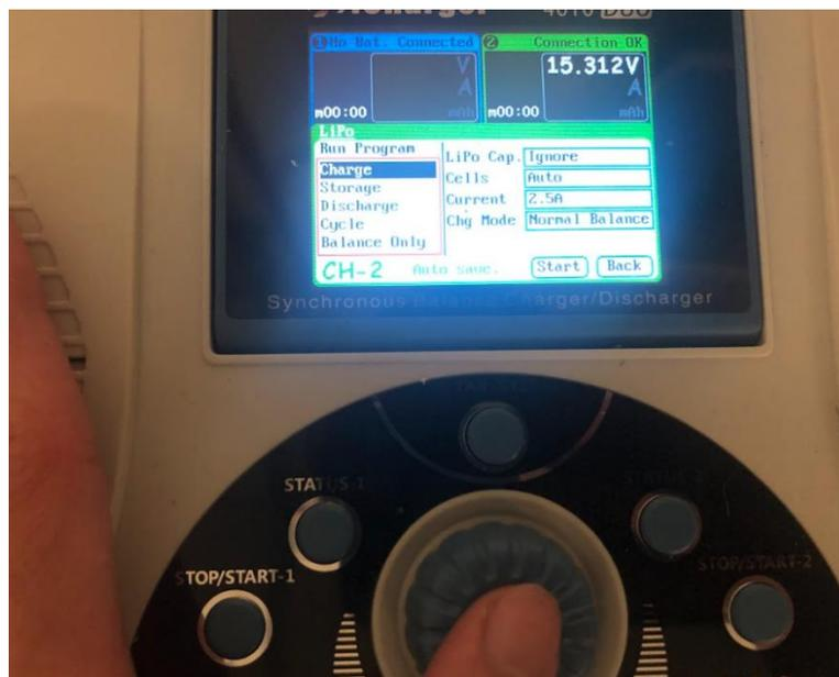
8. If you are satisfied with the Amps, then click the button to confirm: Rule of thumb, safe amps charge is always less than 1\*Ah capacity. Recommend like 0.5\*Ah, better for the battery but double the charge time. Never exceed 12A because of the wire thickness on the power supply.
