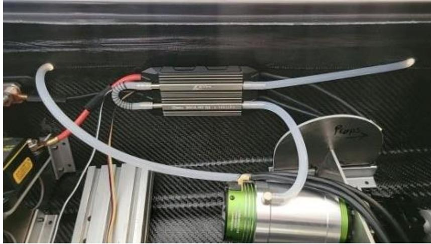
Figure 17: Cooling Loop Between the Motor and ESC
