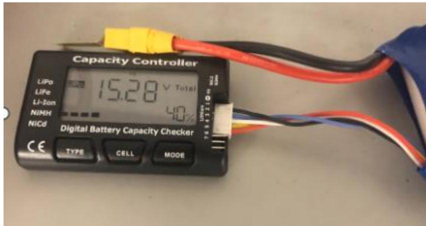
**2. Assess the battery:** Remember LiPo batteries have a minimum voltage of ~3.6V and maximum of ~4.1V in the safe range. To get the nominal voltage, multiply  $3.7 * S$  to get your voltage. You shouldn't go lower than 3.7V because it reduces the lifespan of the battery a little.
