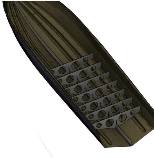
Figure 4: The “Raw” 3D Scan with the BSU Fitted in SOLIDWORKS
