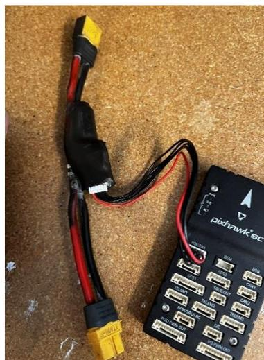
2. Connect the other XT60 connector on the power module to the power board for the battery eliminator circuit (BEC) for the servo motor.
