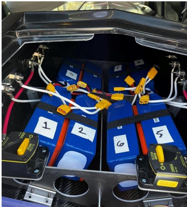
Figure 21: View of the Batteries and Fuses in Position
