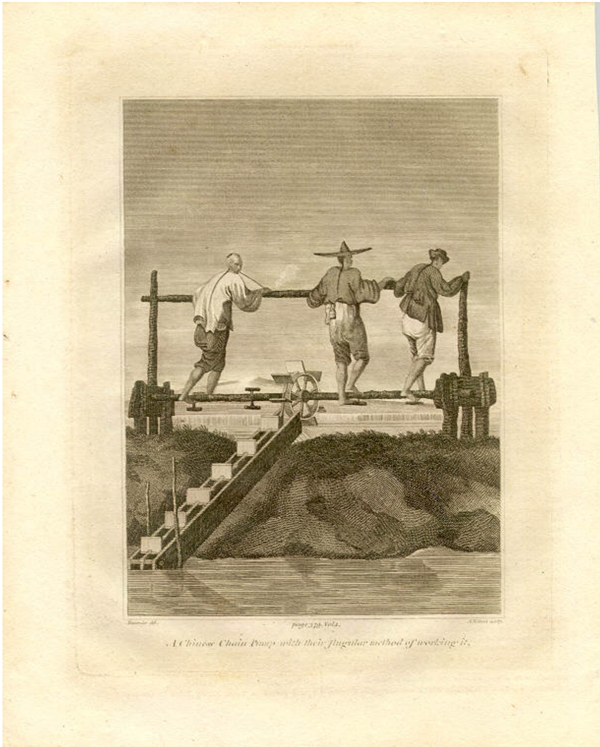
Figure 6. A dragon's backbone tool for irrigation, commonly used in China. It is also known as a square-pallet chain pump. Pumps like these helped farmers reap more rice, but they also increased the labor requirements.
