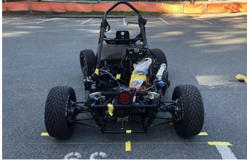
Figure 41: Turning radius test starting setup.
