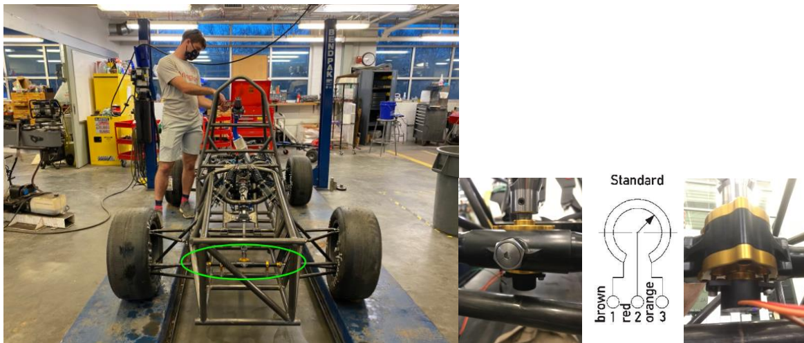
Figure 29: Front steering rack potentiometer placement, close-ups, and wiring diagram.
