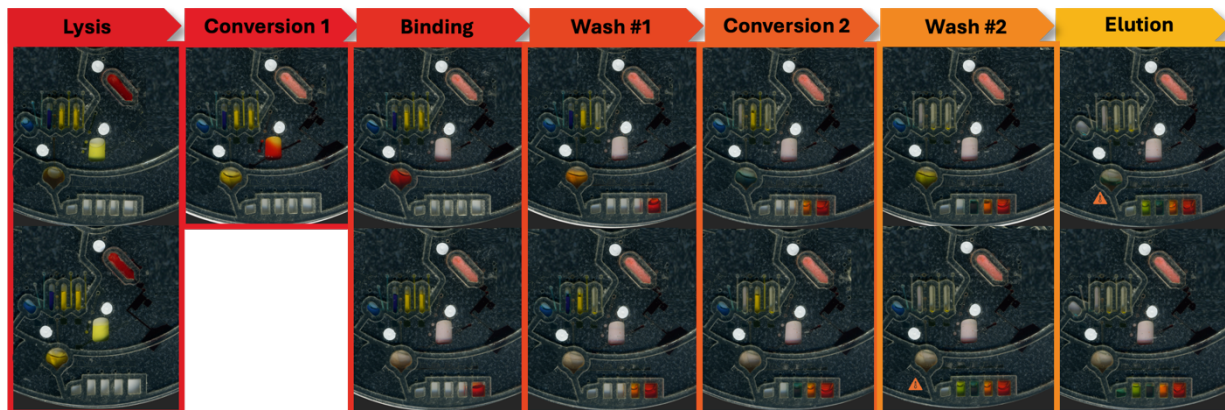
Figure 3-23. Fluidic dye study for integrated disc. Digital scans following the progression of one representative dye study, beginning with direct-from-swab enzymatic lysis and ending with DNA elution of the converted extract.
